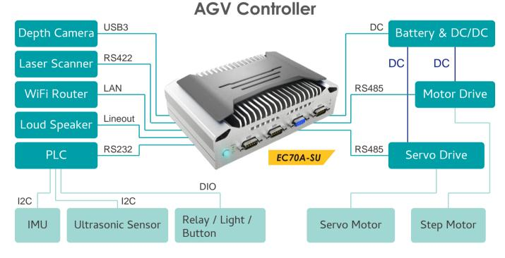
The DFI EC70A-SU/KU series not only bring reliable energy-efficiency, durability, and stability, but also provide a complete I/O interface, ranging from sensors, wireless networks, power supplies, and power systems. It fully meets the need for AMR.
